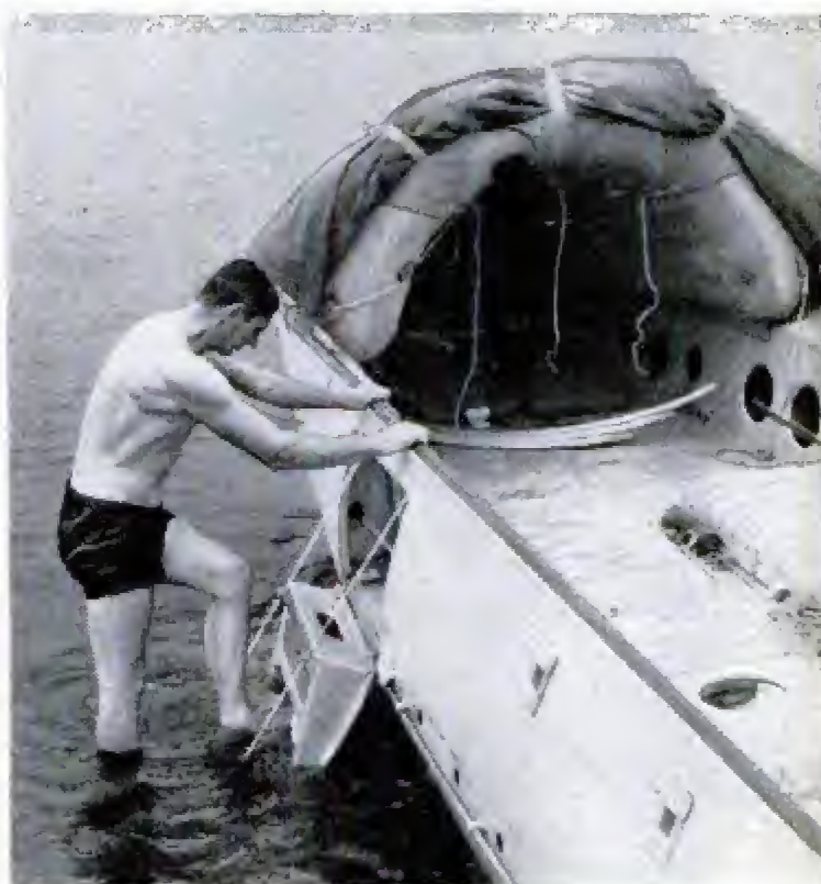
Above, engine is mounted below deck of the craft and can be entirely controlled by unit in hands of engineer. Or, if the passengers are too weak, the operation can be performed from plane by radio. Below, ladder drops into water for survivors
